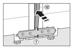
Position the front of the long stainless steel trim in the gap, making sure that it is located above connecting panel i.
